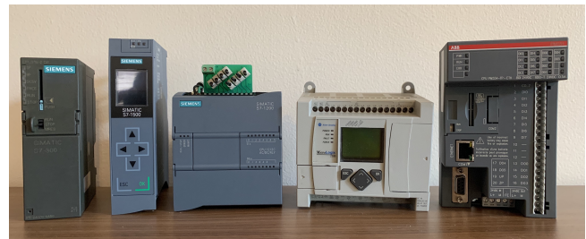
Figure 4: PLCs procured for experimental purposes including, from left to right, Siemens S7-300, S7-1500, S7-1200, Allen-Bradley MicroLogix 1100, and ABB PM554-TP-ETH.
